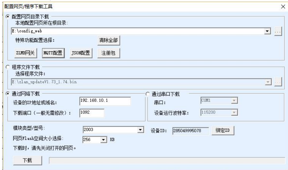
picture18Download configuration file via network port
